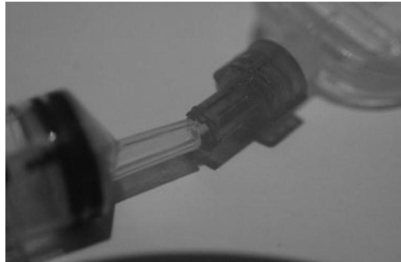
**Figure 5** Failure of attempted cross-connection of a BD syringe male Luer connector into a revised female Neurax<sup>®</sup> connector.
